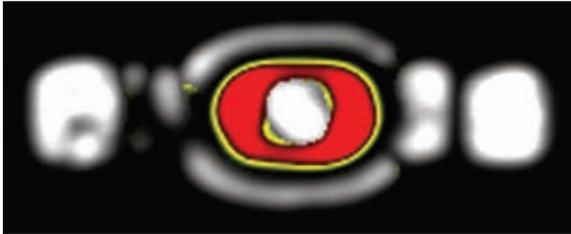
Figure 4. After the lens has been ground flat, topside acoustic imaging of this tiny LED can reveal essentially total delamination of the polymer from the substrate
