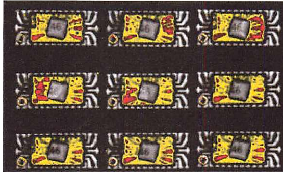
These components were rejected due to excessive lead finger delaminations (shown in red).
