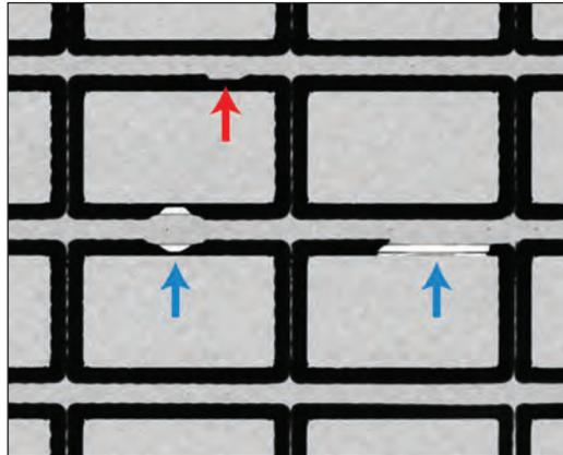
The blue arrows indicate areas where the seal is not bonded to one of its substrates - a condition that destroys the integrity of the cavity. The red arrows indicates an area where the bondline has been thinned laterally. There is no breach, but the bondline may be expected to be thinner and more vulnerable to stresses at this point.
