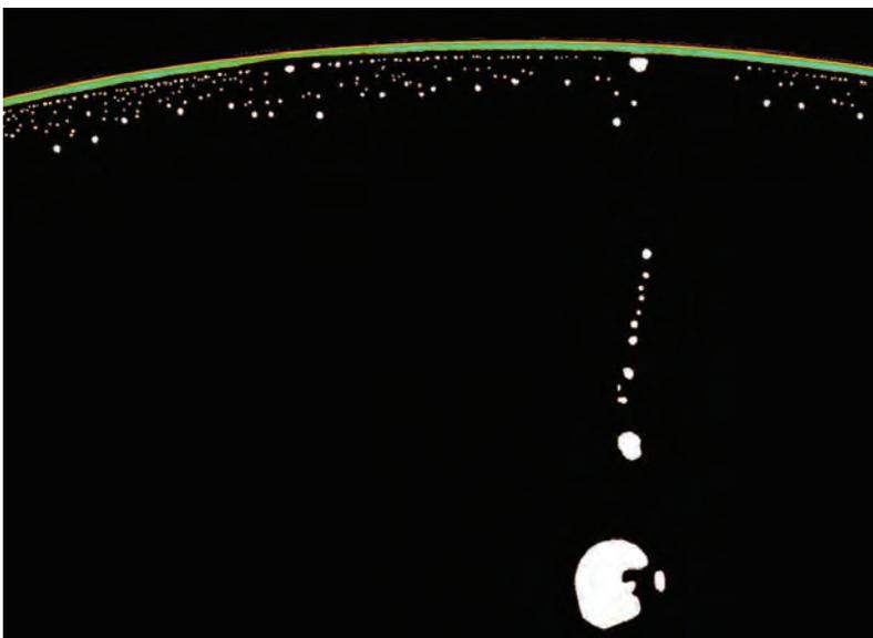
Single wafers that will be used in SOI, BSI and other applications are sometimes imaged before bonding in order to spot surface cracks and subsurface damage. The ultrasound pulsed by
