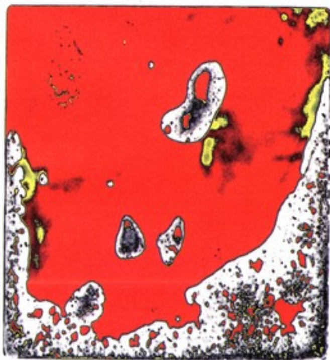
FIGURE 1. Red regions in this acoustic image are voids in the solder bonding the heat sink to an LED.
