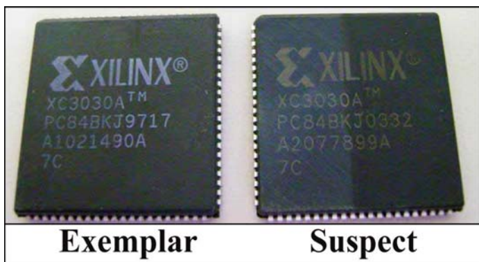
FIGURE 1. New technique removes highly engineered blacktop from counterfeit at right without changing surface of genuine component at left.
