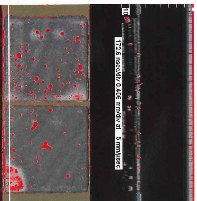
Figure 4: Sectioning through a gray region near the edge of the assembly reveals a lack of solder but many voids.
