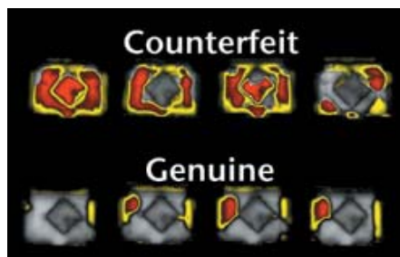
Seen acoustically, counterfeits have larger, more dangerous, inconsistent delaminations. Genuine parts have smaller, less dangerous, and more consistent delaminations..
