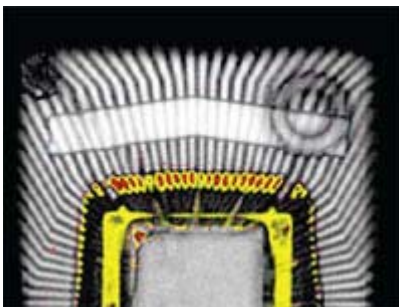
Figure 4. Delaminations (red features) at inner ends of lead fingers, perhaps caused by using a mold compound that does not adhere well to silver.
