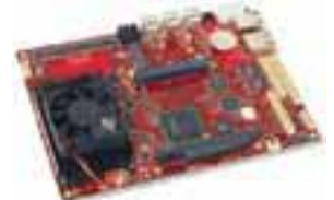
From VersaLogic Corp: Intel® Core™ 2 Duo processor on standard EBX footprint
