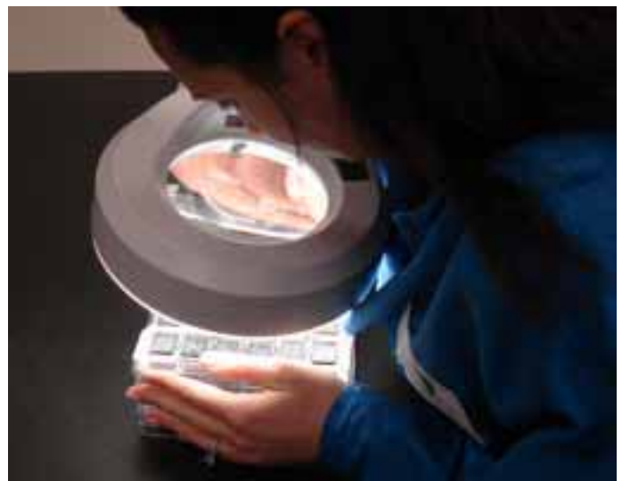
Figure 1. Thorough optical inspection is an initial step in SMT's evaluation of components. [Photo courtesy SMT Corporation]
