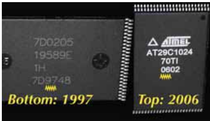
Figure 2. Clumsy re-marking of a counterfeit: the top surface has a manufacturing date of 2006, while the bottom has 1997. [Photo courtesy SMT Corporation]
