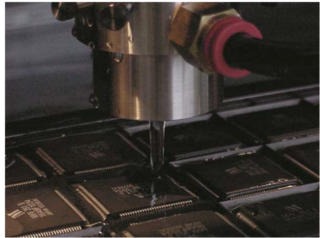
Figure 2. Example of the WaterFall Transducer™ used in C-SAM® automated systems. It provides acoustic imaging without immersion into a water bath.
