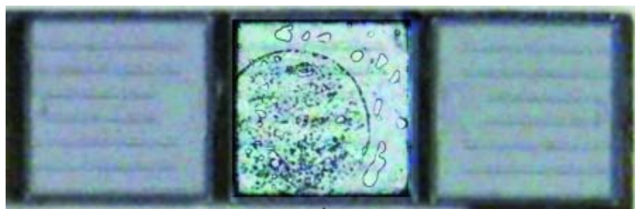
Figure 3: Overlay of the acoustic image of the die attach layer and the optical photo of the die.
