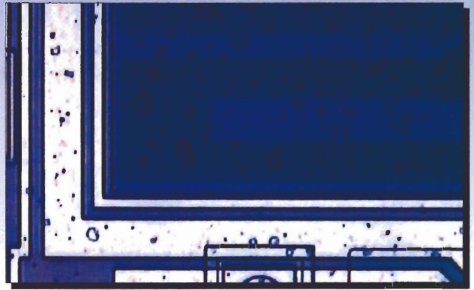
3. Surface of the die after dry decapping. Small irregular areas are the residue of a contaminant. Auger electron spectroscopy showed the presence of silicon, carbon and oxygen, suggesting that the contaminant may have been a silicone. (Source: Riga Analytical Lab Inc.)
