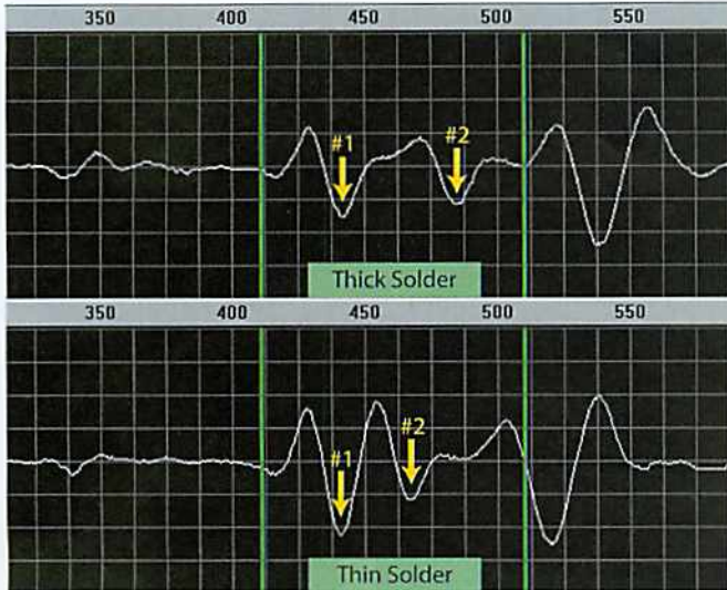
Figure 2: As solder becomes thinner, the peaks representing the heat sink (#1) and the copper (#2) grow closer together.
