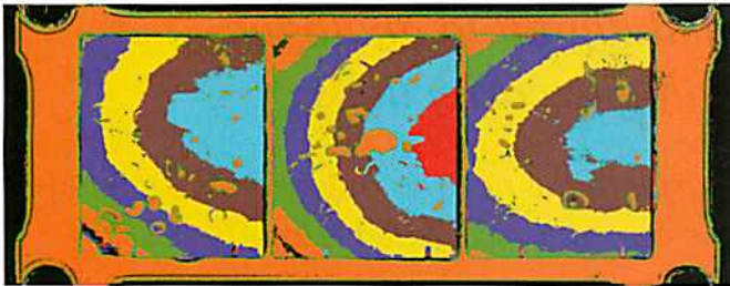
Figure 4: Non-continuous color map makes it easier to identify accept and reject solder thicknesses.
