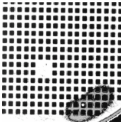
Figure 2: The dark oval in this 50MHz acoustic image is a large void between bonded wafers; the bright spot within the void is the particle, which created the void.
