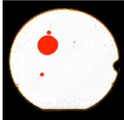
**Figure 2 - Nondestructive acoustic imaging of voids between two bonded wafers. Void size varies greatly, depending on the cause of the void and, if caused by a particle, the diameter of the particle. (Acoustic image courtesy of Sonoscan, Inc.)**
