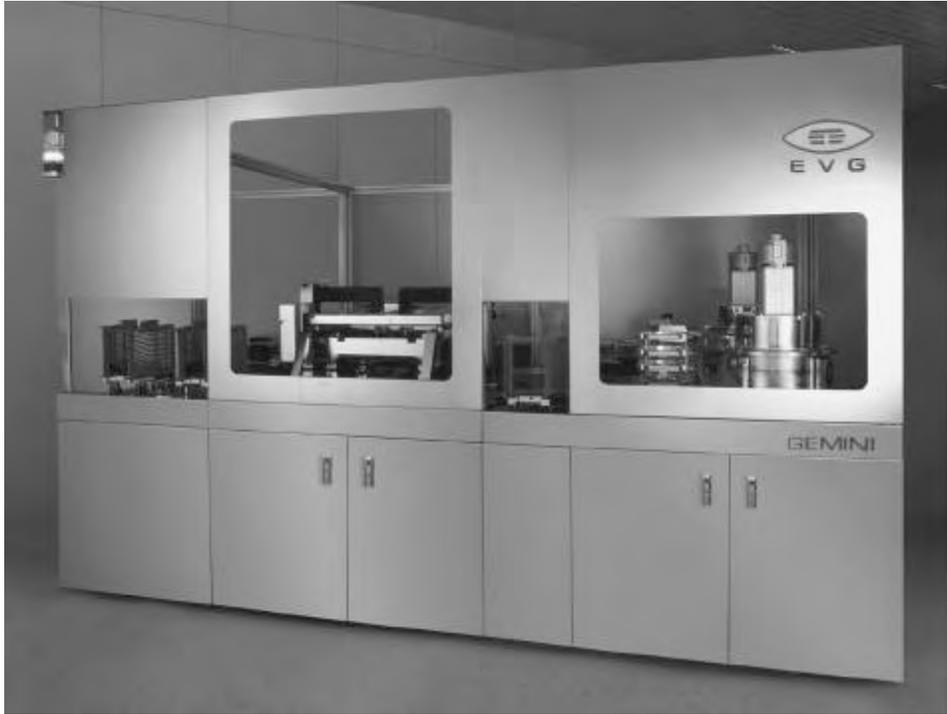
Figure 6 - EVG Gemini automated production wafer bonder. Alignment capabilities include options for bottom side, IR, and Smart View (face to face) alignment. Bonding options range from anodic and thermal compression to SOI. [Photo courtesy EV Group Inc.]
