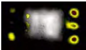
Figure 4. AM image of the bottom side of the PEM device with delamination on three of the four leads, tie bar and the edge of the die.
