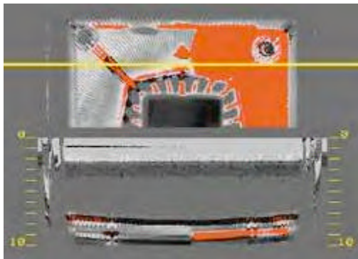
Figure 1. The top half is a normal, planar, “down-looking” nondestructive view into a CSP-like IC package. The bottom half is a nondestructive cross-section through a slice defined by the yellow line in the top half.
