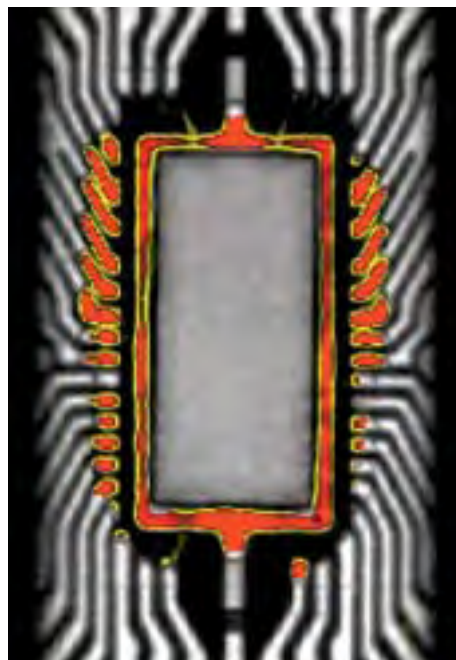
In this acoustic image, some of the delaminations (red) along the lead fingers extend nearly half the distance from the chip core to the exterior. More serious, though, are the delaminations surrounding the die itself
