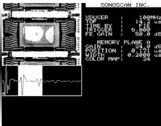
Figure 5B: C-Mode image and A-Scan waveform obtained at 100 MHz.
