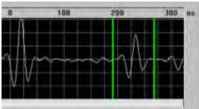
Figure 3: A-scan displaying typical waveforms (pulses) in the time domain.
