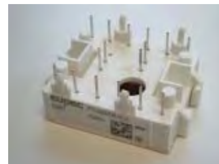
The Easy1 housing offers a well suited module concept for a compact and cost-effective integration of power
