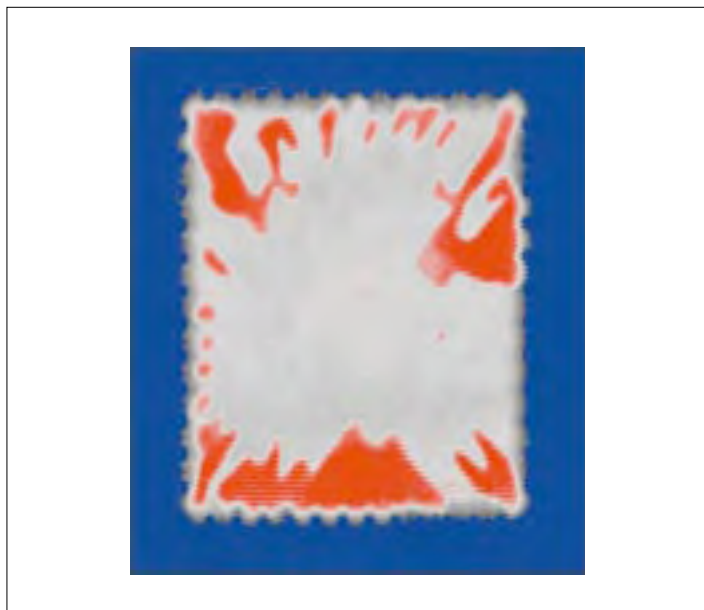
Delaminations (red areas) between the cured underfill and the die face, imaged acoustically after stress testing.
