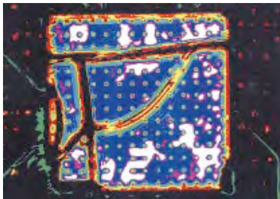
Figure 3: The acoustic image of a device reveals how the lack of underfill in certain areas causes a device to crack into several pieces.
