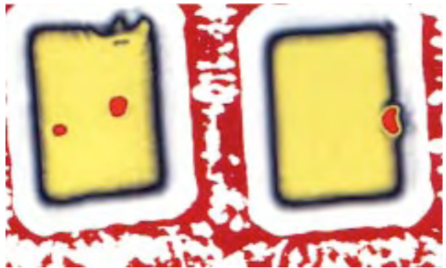
Figure 2: Acoustic imaging of microSMTs at 180 MHz shows small de-laminations (red) between the silicon and epoxy layers.
